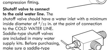
**NOTE:** A Self Piercing Saddle Type Water Valve should not be used.
